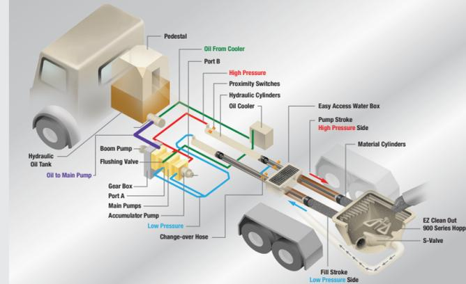
Unlike an open loop system, the oil flows freely without passing through any unnecessary valves that can generate heat. Thus, the closed loop requires far less oil to run the system, as a larger reservoir is not necessary to cool all of the oil. In addition, return oil can be cycled directly through the main kidney filter instead of going back to the tank, keeping it in the filtered state preferred by the hydraulic components for long life and dependable operation.
